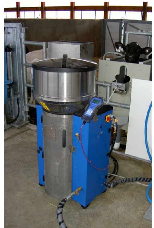
Fig. 1: Computer-controlled calf feeder with feeding station
